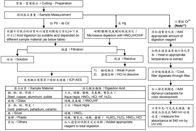
Note\*\*: (1) 針對非金屬材料加入鹼性消化液,加熱至 90~95℃萃取. / For non-metallic material, add alkaline digestion reagent and heat to 90~95℃.
