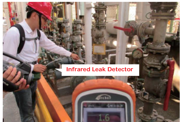
Voluntary checkups are carried out regularly to detect the leaking source in the plant
