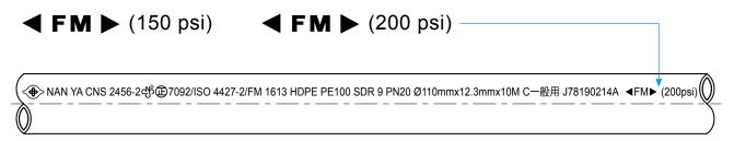
Marking of Ø100mm~Ø630mm PE Pipes for underground fire protection (for example Ø110mm SDR 9)
