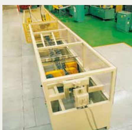
靜水壓重複彎曲試驗 Flexural Test for Hydrostatic Pressure
