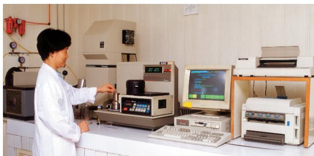
● 动态机械黏弹仪 Dynamic Mechanical Test
