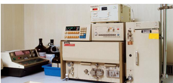
● 核磁共振光谱仪 Nuclear Magnetic Resonance Spectrometer
