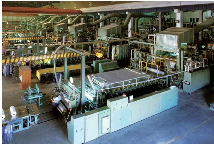
●硬质胶布生产设备 Production equipment of rigid PVC film
